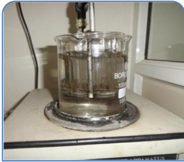
Disintegration test of KVR
